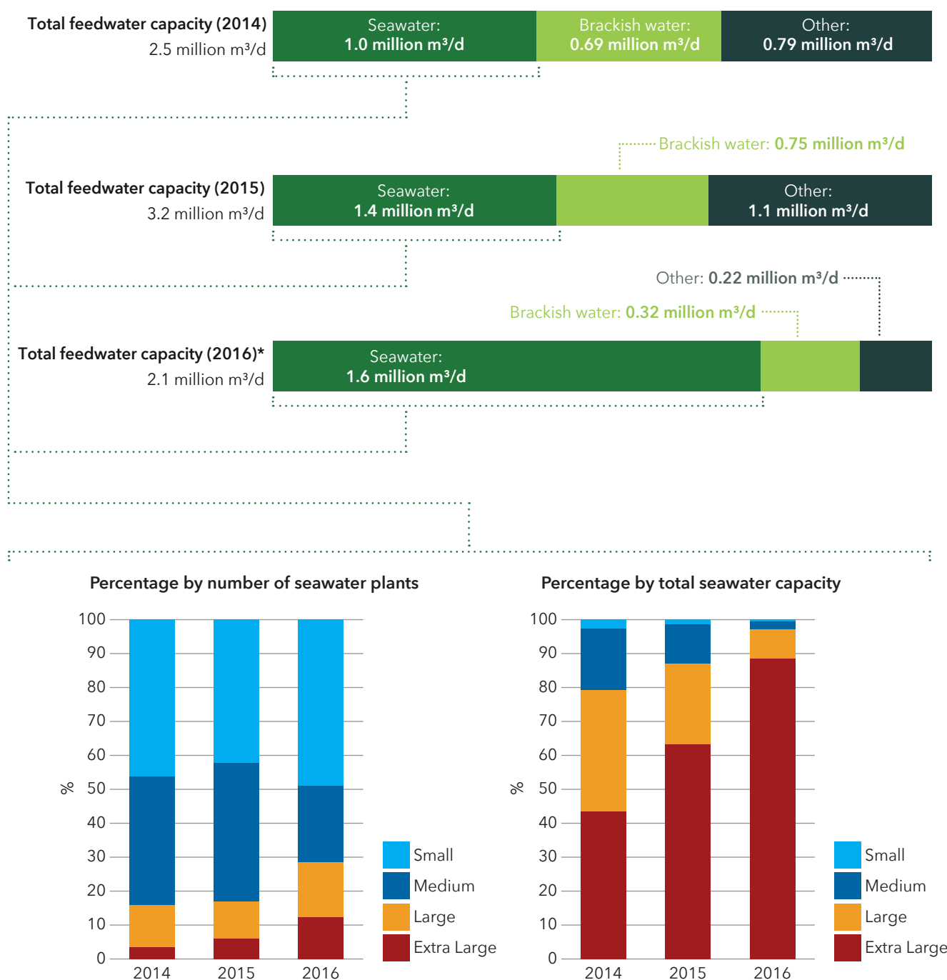
FIGURE 6: CAPACITY BY FEEDWATER TYPE AND SIZE DISTRIBUTIONS OF SEAWATER DESALINATION, 2014-2016
